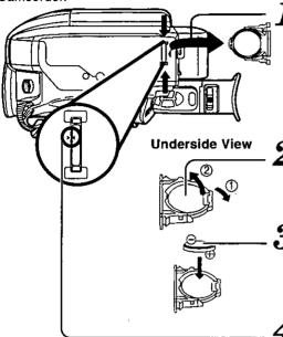
While pinching the stopper tabs, pull the Battery Tray out of the Battery Compartment.
