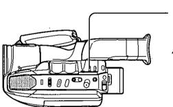
**1** Press HIGH SPEED SHUTTER while recording.
