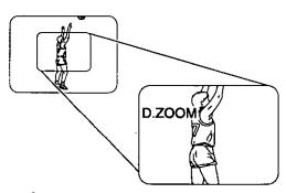
1 Press the DIGITAL ZOOM button on top of the Camcorder to select D.ZOOM mode.
