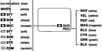
■ To create more effects: You can stop the fade at any time by pressing the MODE SEL button (other than BLACK, WHITE, and RANDOM modes). Pressing the FADE button will continue the fade. Pressing the MODE SEL button will cancel the fade.
