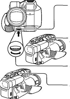
Press MANUAL FOCUS so that "MF" (Manual Focus) appears in the EVF.
