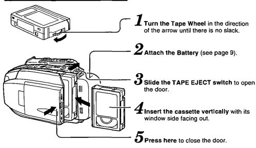
• To remove the cassette, slide the TAPE EJECT switch.
