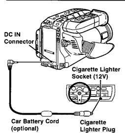
Connect a PV-C16 Car Battery Cord (optional) to DC IN on the Camcorder.
