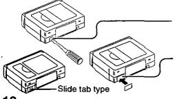
**1** To prevent accidental erasure, break off the tab with a screwdriver. (If slide type, slide tab open.)
